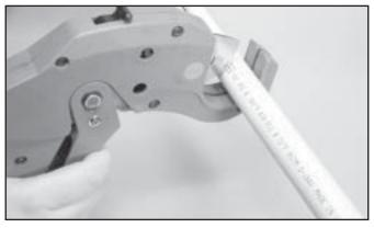
Be careful not to split the tube if using a ratchet-type cutter, especially in temperatures below  $50^{\circ}F$ . If any damage or cracking is evident, cut off at least 2'' of the tube beyond any visible crack.
