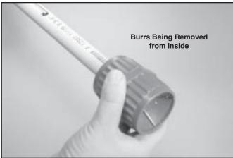
A slight bevel must be placed at the end of the tube, as shown below. A slight bevel will ease the entry of the tube into the socket and minimize the chance of cement being wiped off the fitting.
