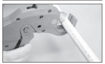
Be careful not to split the tube if using a ratchet-type cutter, especially in temperatures below 50°F. If any damage or cracking is evident, cut off at least 2" of the tube beyond any visible crack.
