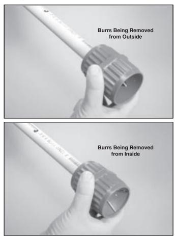
A slight bevel must be placed at the end of the tube, as shown below. A slight bevel will ease the entry of the tube into the socket and minimize the chance of cement being wiped off the fitting.
