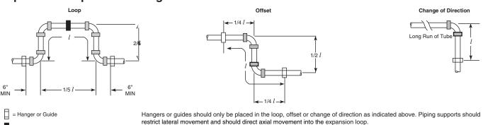
Coastline EverTuff CPVC, like all piping materials, expands and contracts with changes in temperature. The coefficient of linear expansion for CPVC is 3.2 X 10 – 5 inch/inch-°F. A 25°F change in temperature will cause an expansion of 1" for a 100-ft straight length. For most installation and operating conditions, expansion and contraction can be accommodated at changes of direction. Based on the following chart, an offset or loop is required on a long, straight run.
